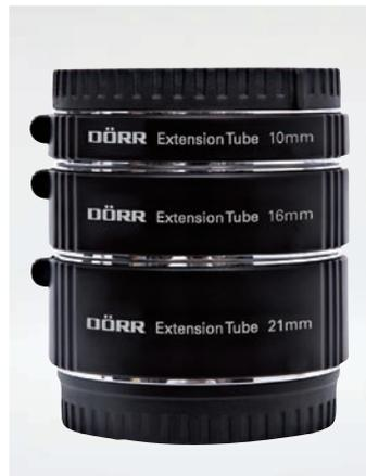
For great macro shots with DSLM cameras. The extension tubes can be used individually or combined. They are mounted between the camera and lens. They reduce the minimum distance of the camera lens and thus increase the ratio for close-up photography.
